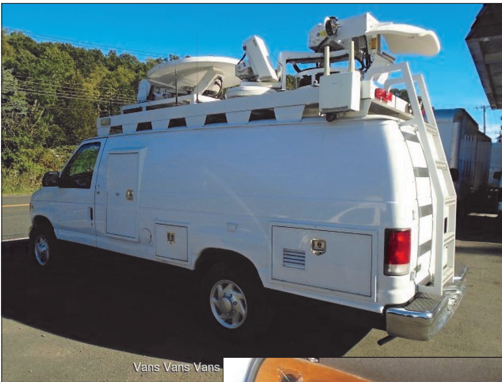
Drivers side rear view. Air compressor is behind door closest to you. On top closest to you is the framework holding the terrestrial dish and camera, all mounted to the pneumatic mast. The ring for the coiled cable bundle is just visible.
